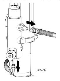
5. Using a wrench, loosen filter housing fitting (110) and remove housing from pump.
